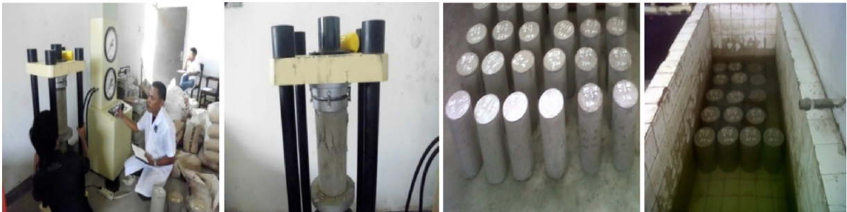
Fig. 1. Compressive strength test process.
